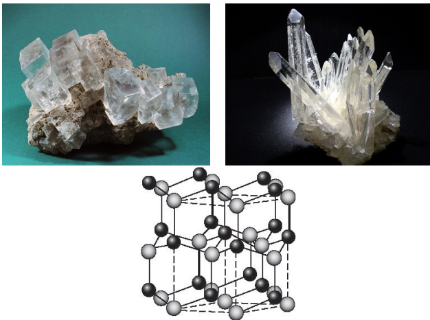
Figure: Crystals of ordinary salt \text{NaCl} , of quartz \text{SiO}_2 , and an example of crystalline lattice ( \text{SiO}_2 - wurtzite). The interatomic forces impose the shapes and the geometry of solid bodies.
